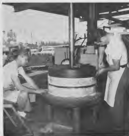
VARIETY OF Machine Shop tasks includes babbiting as performed here by H. Kelly, left, and S. de Cuba. Babbiting serves as a wiper ring for Edeleanu Plant compressor piston. E VARIEDAD di trabaoan den Machine Shop ta inclui "babbiting" cu cual H. Kelly, robes, y S. de Cuba ta trahando aki. Babbiting ta sirbi como un wiper ring pa piston di compresor pa Edeleanu Plant.
